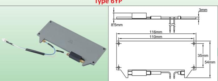
Immediately below the level of the transparent window, the warm air flow it generates prevents from condensation on the window and keeps an optimum ambient temperature for the control devices in the housing. It has a wide aluminum heat exchanger to reduce its surface temperature and a miniature snap-action thermostat limits the temperature inside the cabinet.
